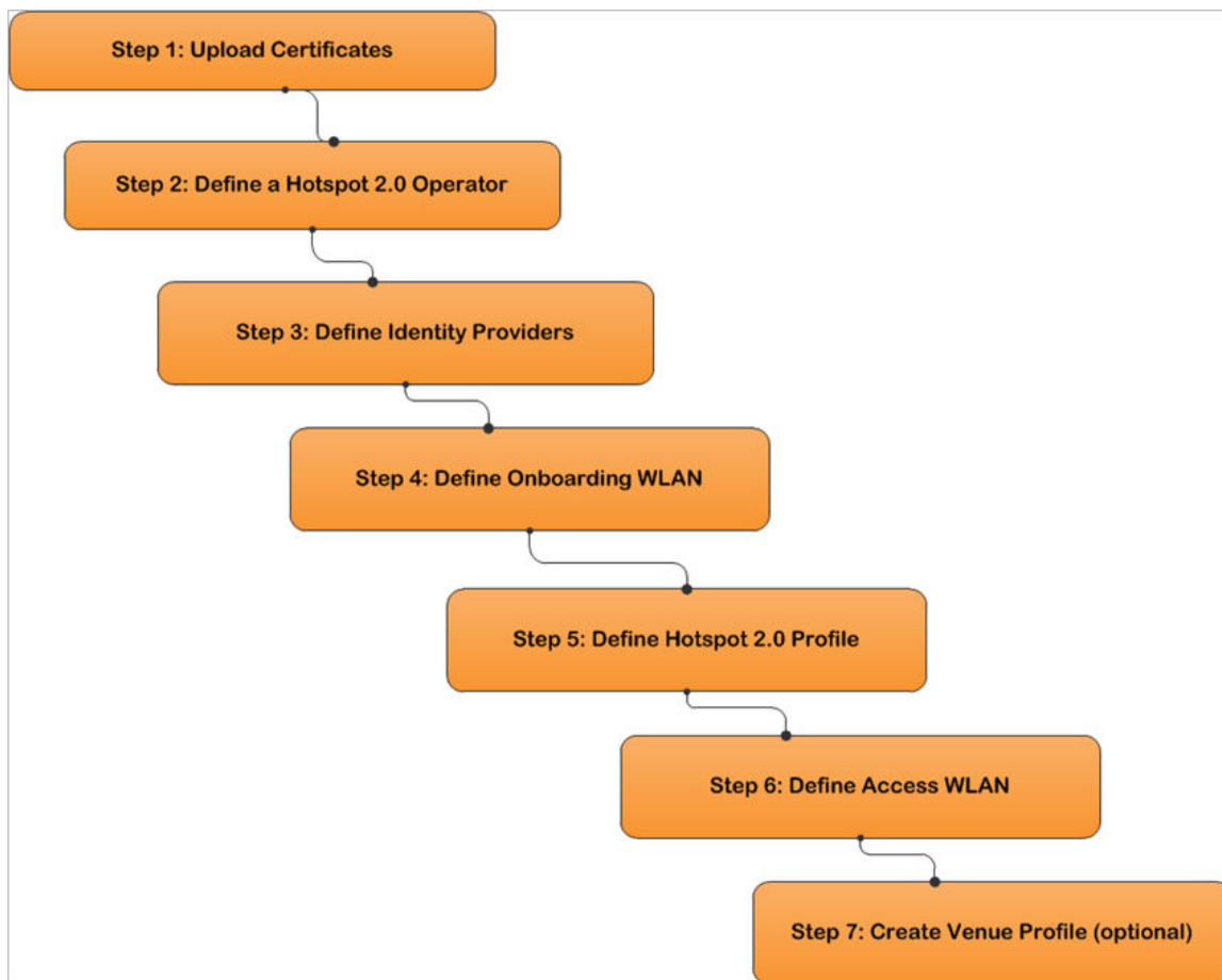
FIGURE 3 Hotspot 2.0 Configuration Flow
